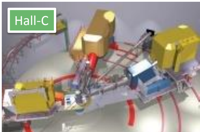
Super High Momentum Spectrometer (SHMS) at high luminosity and forward angles
