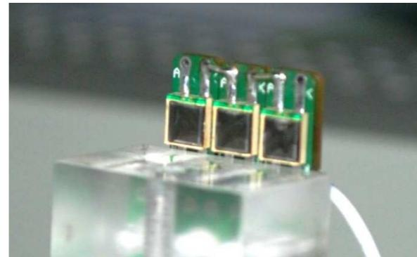
Active area:  $3 \times 3\text{mm} \times 3\text{mm} = \mathbf{27\text{ mm}^2}$
