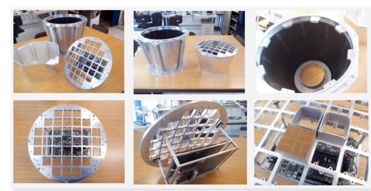
Photo-sensors = SiPMs (S11828-3344M, other sensors under test for the mini-array)
