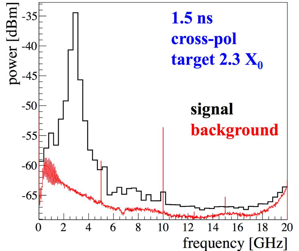
main line at  $f_{\text{LINAC}} = 2.85 \text{ GHz}$
