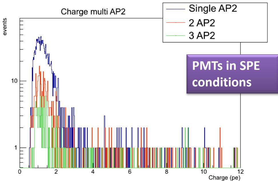
Differently to 10-inch PMT , in 3 inch PMT multiple AP2 have a charge mainly of spe. Multiple AP2 show lower fractions in confront of 10-inch PMT.
