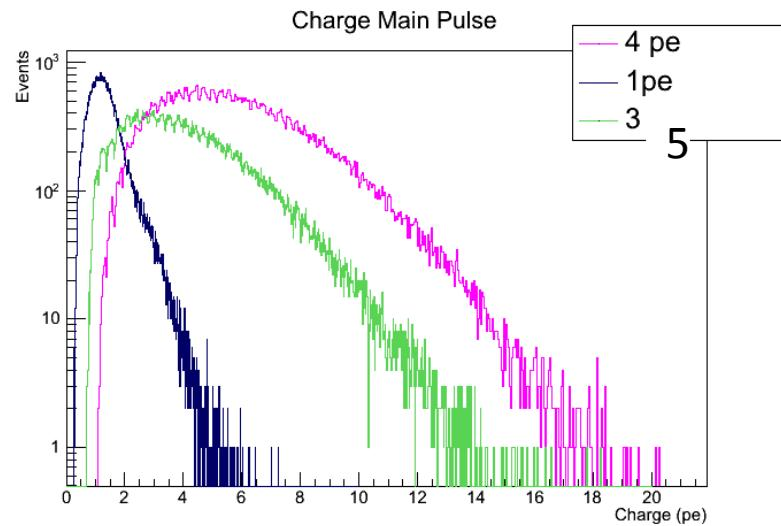
Changing PMT conditions from 1 to 5 pe, TTS is reducing and Pre pulses and delayed fractions became lower
