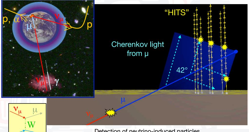
Detection of neutrino-induced particles through the observation of Cherenkov light
