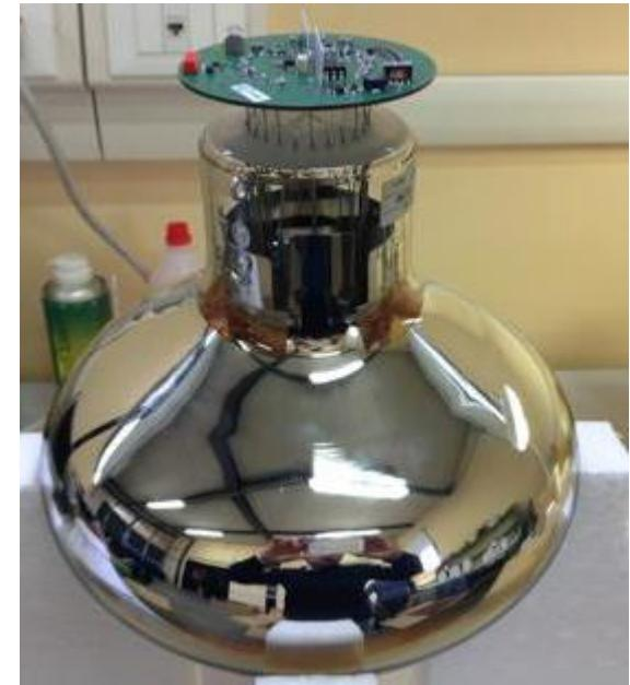
Hamamatsu 10-inch PMTs with the ISEG base soldered
