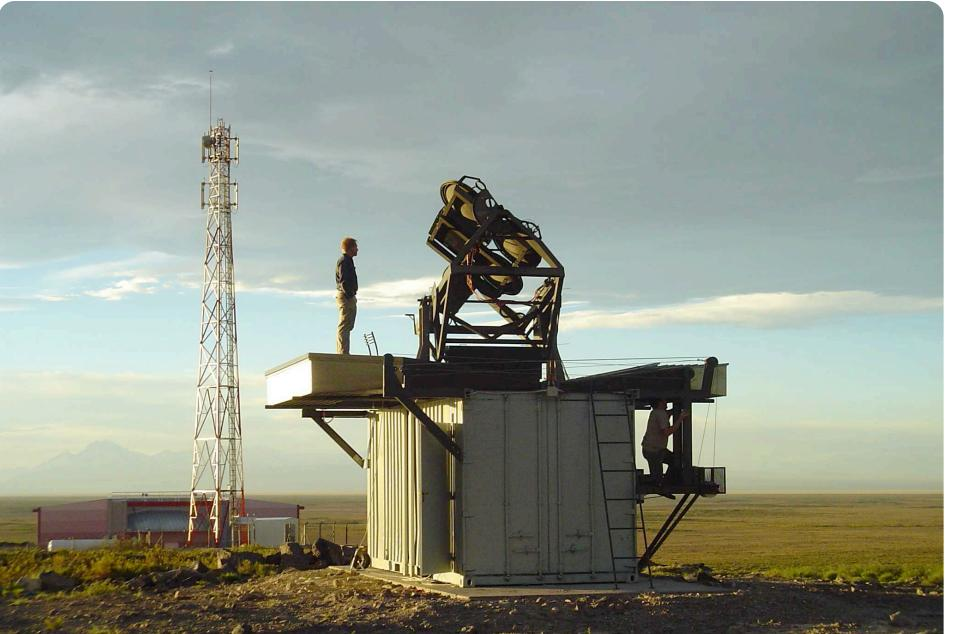
4 parabolic mirrors (one for the short range,  $\emptyset = 20$  cm; three for the long range,  $\emptyset = 80$  cm).
