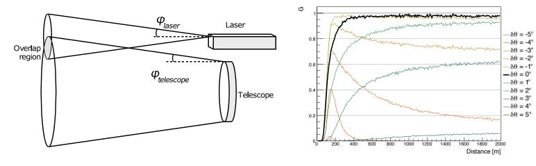
Horizontal shots are also used to extract the aerosol extinction coefficient at ground  $\alpha_{aer}(0)$ .
