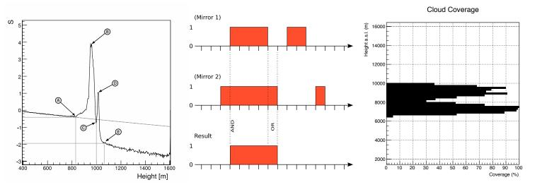
The lidar central control selects these events by applying different quality cuts. For those events that pass the cuts, it orders the lidars to shoot simultaneously along the reconstructed shower track. Fluorescence detectors are vetoed during this operation.
