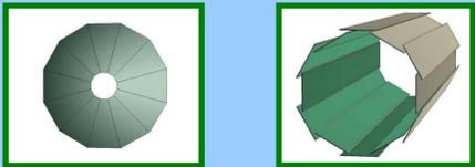
one layer of the VXD endcaps    one layer of the VXD barrel
