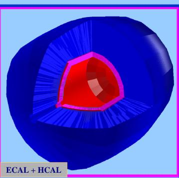
**Dual Readout Electromagnetic Calorimeter (ECAL)**
