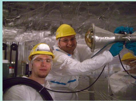
Six more PMTs just below the cryostat will complete the GERDA muon veto. The PMTs are encapsulated in housings of stainless steel with a PET window at the front. To protect the PMTs against the water, the contacts of the voltage divider are protected with polyurethane and silicone. Long-time tests (more than one year under water) show that the capsule is water tight.
