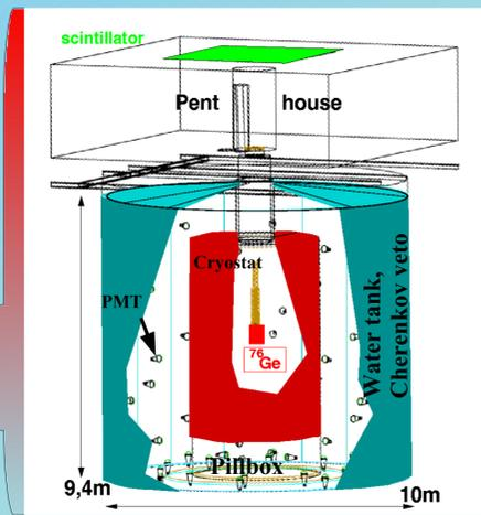
GERDA-geometry, with final PMT distribution, used for the Monte-Carlo-simulations, implemented in the MaGe framework.
