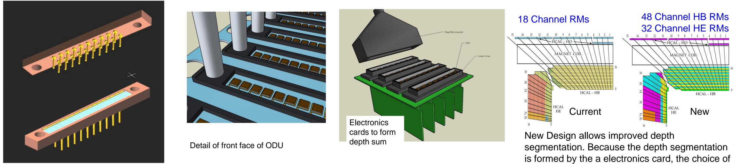
New Upgrade will use "Strip SIPMs, 18 1mm SIPMs in ceramic package. Connect to optical cables from HCAL The HCAL ODU is replaced by an "EDU" where single SIPMs per optical fiber are ganged together into depth segments, then digitized
