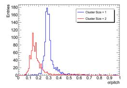
Spatial resolution for BM chambers obtained from a gaussian fit of the residual distribution normalized to strip pitch, in the case of clusters of size 1 (blue line) and size 2 (red line). As expected cluster of size 2 show a better resolution due to the small region in which the particle crosses the detector.
