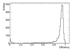
Panel efficiency for BM chambers at working point (HV 9.6 kV,  $V_{th} = 1.0 \text{ V}$ ).
