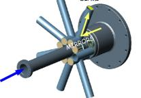
Cherenkov light can be redirected far from the guartz window using mirrors to:
