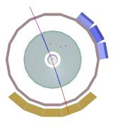
Cosmic muons reconstructed as independent tracks in upper and lower halves of TPC
