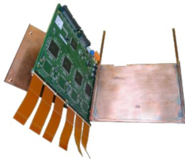
Water cooled copper envelope for front-end card
