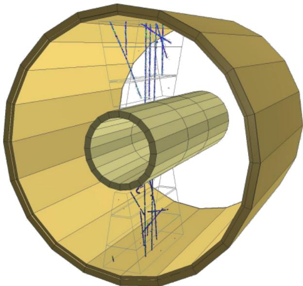
First cosmic tracks detected by the ALICE TPC during the pre-commissioning on the surface in 2006. The fraction of the electrical power and of the corresponding water-cooling plant available at the test site was sufficient for operating only two sectors at a time.
