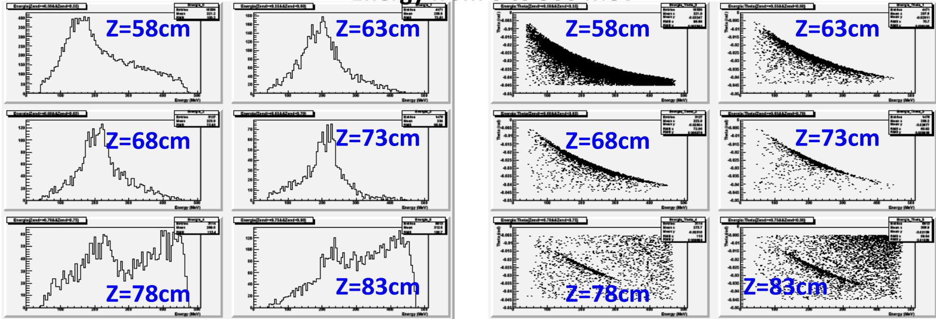
electron energy vs. beam escape position  $Z$  with respect to the interaction point
