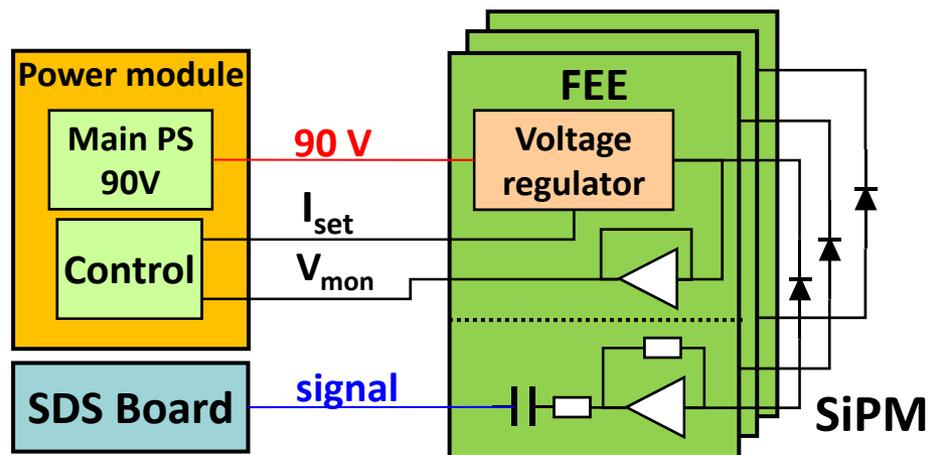
We coupled this front-end electronics to Hamamatsu SiPM (MPPC) S10362-33-050C with 3600 pixels, 3x3 mm<sup>2</sup> active area
