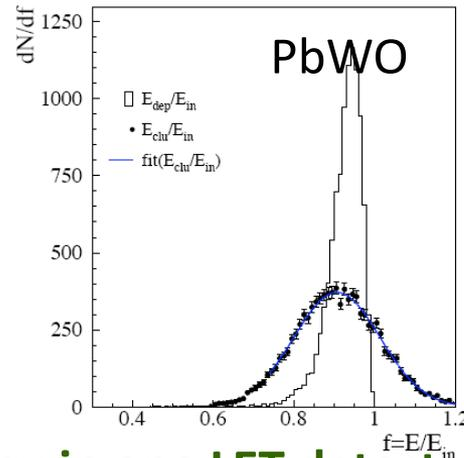
Deposited and detected energy in one LET detector, averaged over the impinging off-energy beam particles.
