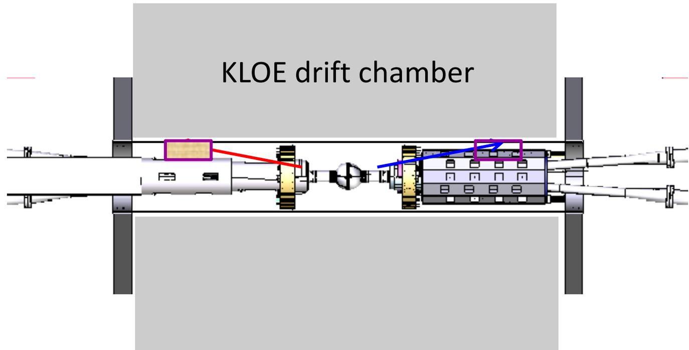
Electrons and positrons escape from the beam pipe with  $11^\circ$  angle
