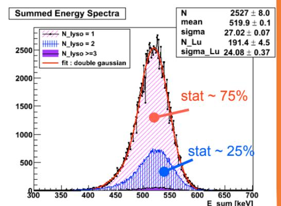
Summed energy spectra of the lyso crystals in the matrix, corresponding to different crystal multiplicities (N\_lyso = 1, 2, 3 or more). The asymmetry in the photopeak is explained by the Lu X-ray escape peak and represented by a double gaussian fitting function.
