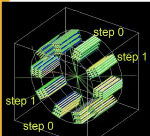
Screenshot of the AXPET simulations in a 5-steps acquisition. Each step corresponds to two modules used in coincidence.
