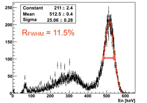
Typical energy distribution of the photons detected in one crystal, when the matrix is exposed to the 511 keV annihilation photons from the <sup>22</sup>Na source.
