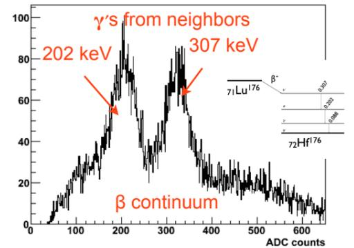
Typical measured spectrum of intrinsic radioactivity of a single LYSO crystal in a matrix arrangement.
