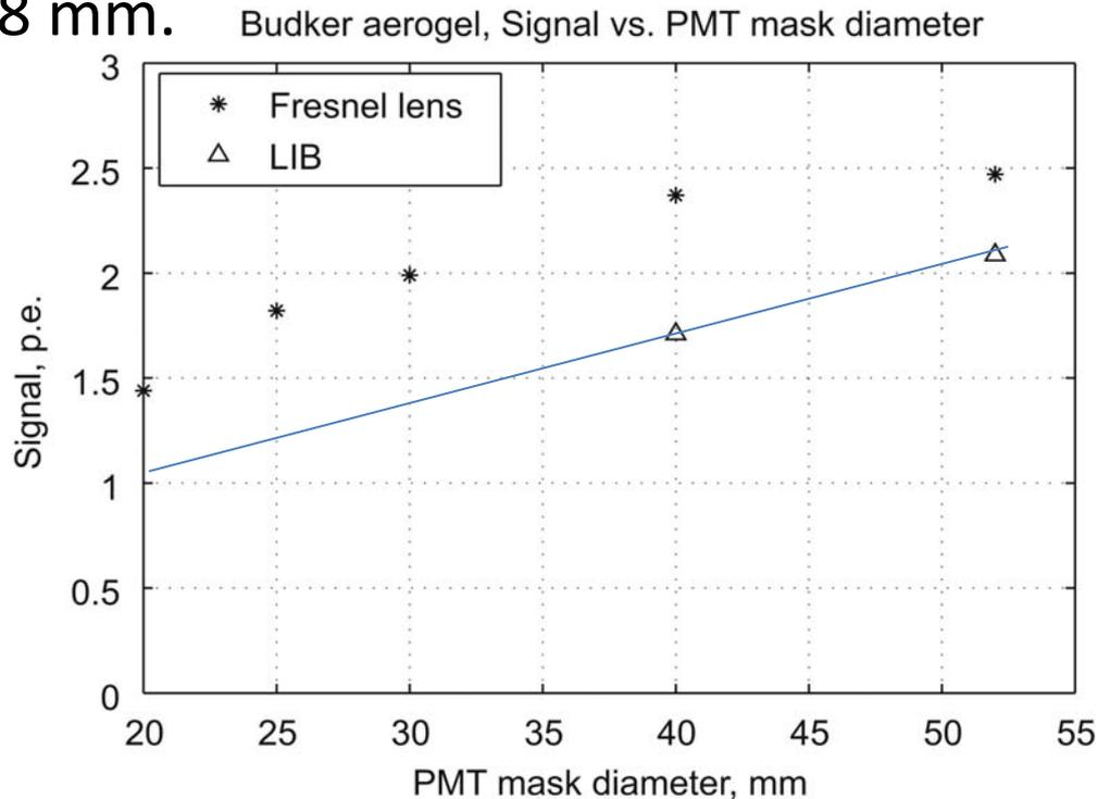
Signal collected with Fresnel lens and LIB, aerogel  $n=1.015$ , as a function of the PMT effective diameter. The size of the Cherenkov ring for this aerogel is 25 mm.
