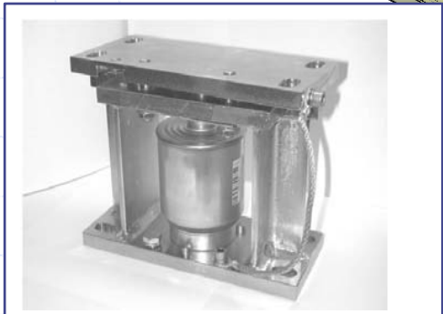
load cell accuracy < 0.02%
