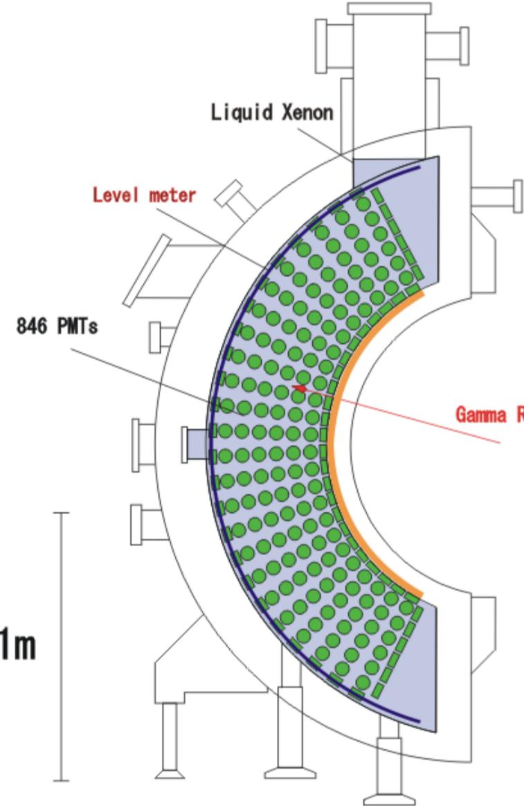
We use 850l liquid xenon as a scintillator. The scintillation light is detected by 846 PMTs surrounding the active volume of LXe. LXe properties enable us to measure the energy, timing and position of incident  $\gamma$ -ray at the same time with required resolution
