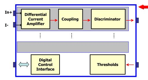
General architecture of the chip: Eight channels with independent adjustable thresholds.
