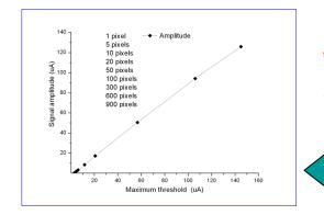
Dynamical range and linearity for thresholds regulation of the chip: Simulation results vs measurements.
