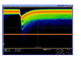
Timing results: Time distribution obtained with a fixed pulse amplitude corresponding to about 27 equivalent hit pixels.
