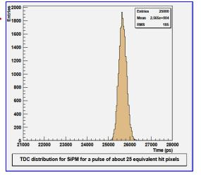
Cosmic ray test: with 1x1mm<sup>2</sup> Hamamatsu SiPM coupled with a small BC418 plastic scintillator.
