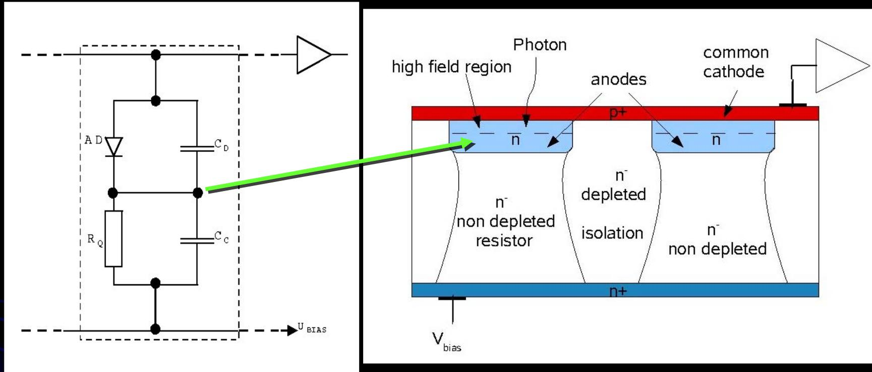
Front side  $p^+$  cathode and backside  $n^+$  region are common for the entire array
