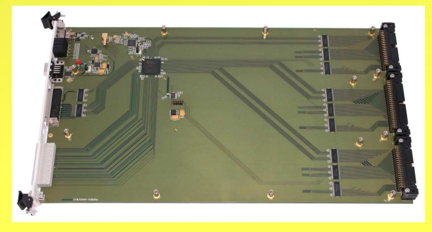
Tester board is practically a mirror of the LB. It makes possible to do the testing in the rack. The inputs of the LB are outputs of the Tester and the other way around. There is one Xilinx Spartan 3 FG 456 FPGA on the tester board circuit to perform the testing. Communication to PC and controlling of the test is made with RS323 connector and LPC2106 micro controller. Twelve LEDs on the tester are giving fast information about test results.
