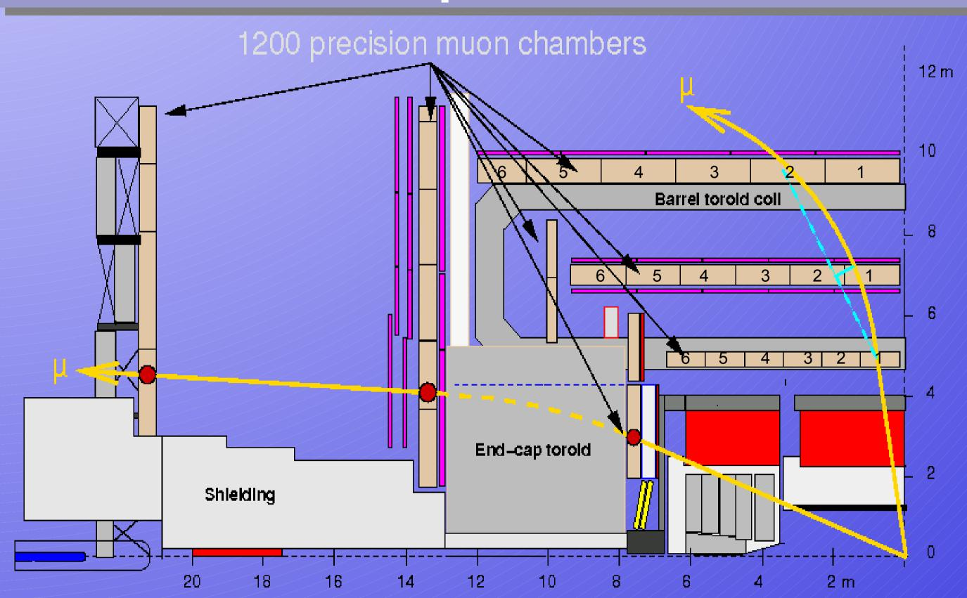
Air core toroid magnet to minimize multiple scattering: barrel: B = 0.15 – 2.5 T end-caps: B = 0.2 – 3.5 T
