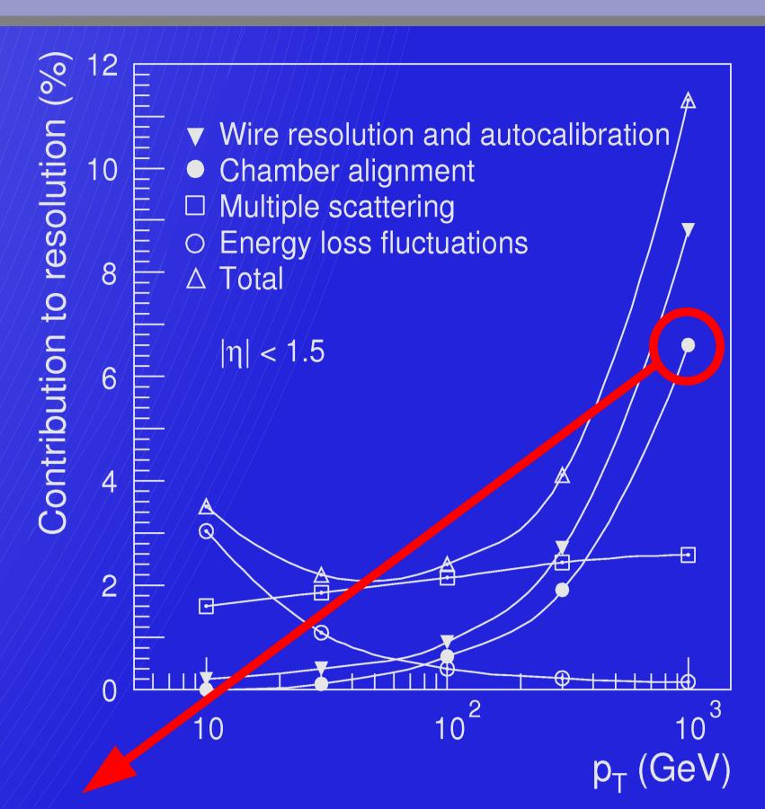
Muon chamber alignment accuracy: ~30 µm
