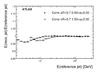
Example of calibration using H1-method, applied on a sample of QCD jets.
