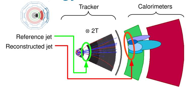
Reference jet : built from all the stable particles (except  $\nu$  and  $\mu$ ) coming from the quark (or the gluon) fragmentation.
