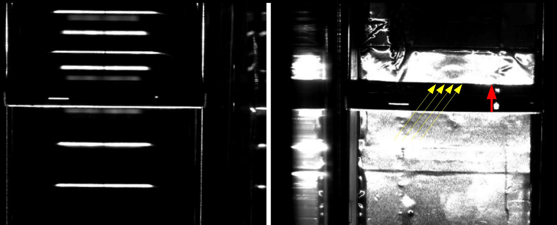
Pictures of a tray taken by the BMS vision system before (left) and after (right) insertion of bricks. The shadow of the tray visible on the brick surface is used to compute the distance of the brick with respect to the tray border.
