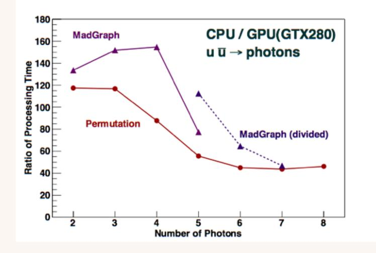
Large reduction of process time / event loop from CPU to GPU (single precision)
