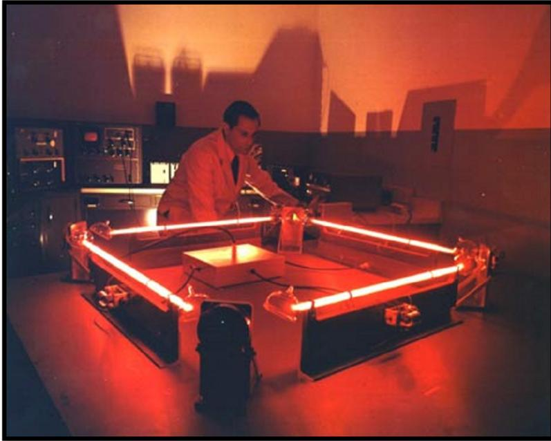
While the first laser gyro did not unlock on the rotation rate of the Earth and had to be spun to demonstrate gyroscope functions...
