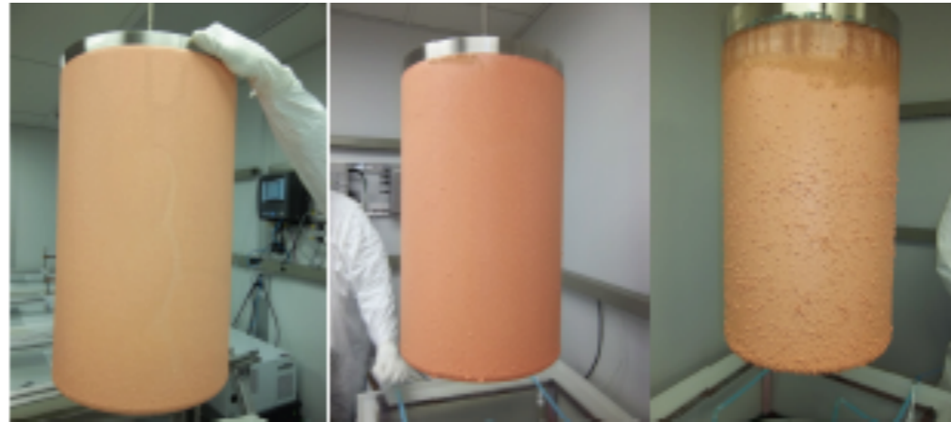
Inspection of EF copper on mandrels
