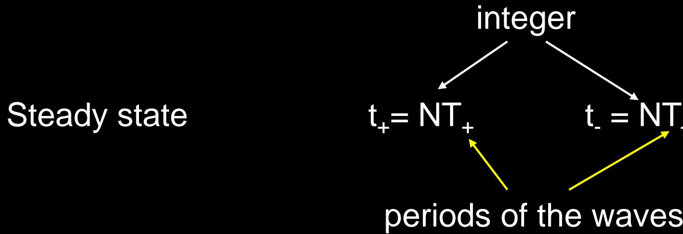
$$\Delta t = N(T_+ - T_-) = N\left(\frac{1}{\nu_+} - \frac{1}{\nu_-}\right) = N \frac{\Delta\nu}{\nu_+ \nu_-}$$
