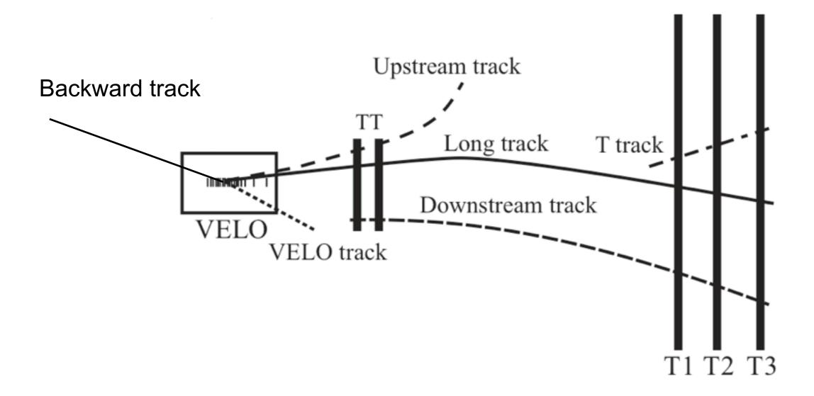
**VELO:** surrounds the interaction point - high reconstruction efficiency **Long Tracks**: Relative momentum uncertainty 0.4-0.6% **IP resolution**: 20µm IP for p > 2 GeV,  $p_T > 200$  MeV
