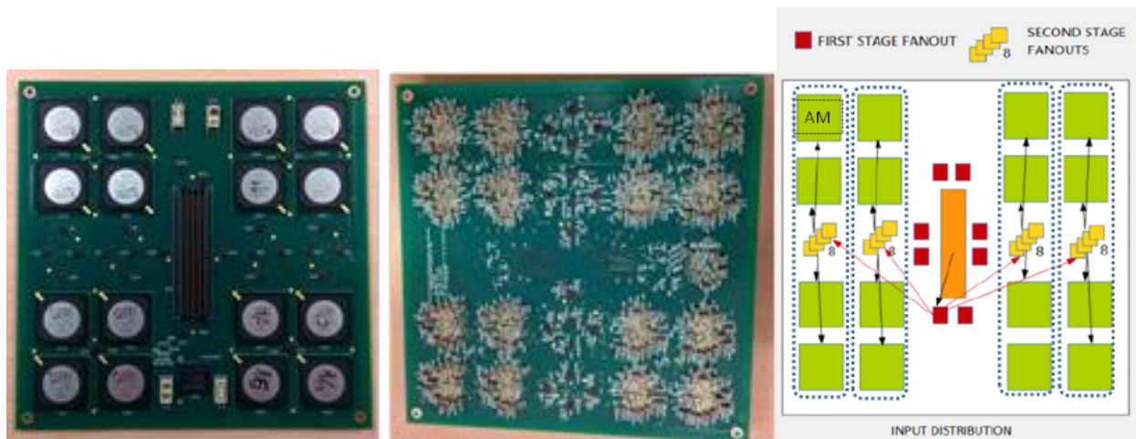
Figure 0b: The LAMB and the input data distribution to AM chips.
