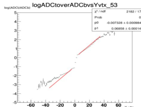
For central slats (52,53,54) with the hole and for other problematic slats (51 and 151) in which a discontinuity seems to be present, we implemented a discontinuous fit above and below the gap.
