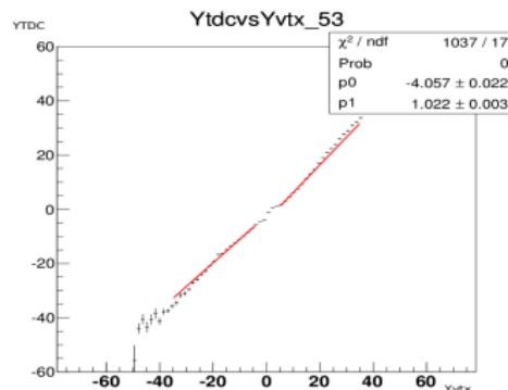
For central slats (52,53,54) with the hole, we implemented a discontinuous fit above and below the gap.
