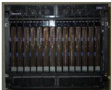
IBM blade H - (14/14) 2 socket - 4 core RAM 32GB
