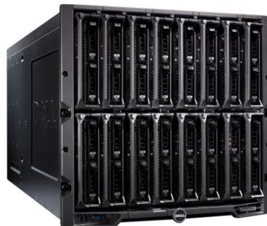
Dell blade M1000e (16/16) 2 socket - 4/6 core RAM 48GB
