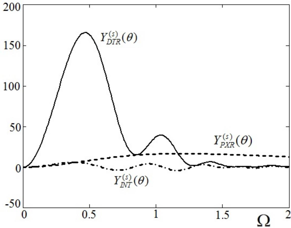
**Fig. 17.** Angular density of PXR, DTR and their interference term . The curves are built for such values of parameters:  $\Gamma = 0.5$ ,  $\chi'_c / \chi'_0 = 2$ ,  $B^{(s)} = 3$ ,  $\varepsilon = 3$ ,  $\nu^{(s)} = 0.8$ ,  $a/b = 1.676 \cdot (2m+1)$ ,  $c/b = 0.335 \cdot (2n+1)$ , which correspond to the conditions of constructed interference
