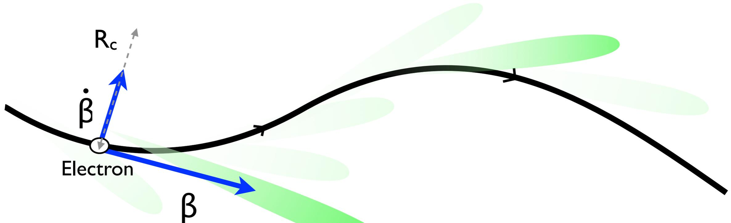
To efficiently produce X-ray radiation we need relativistic electrons undergoing oscillations (synchrotron radiation)
