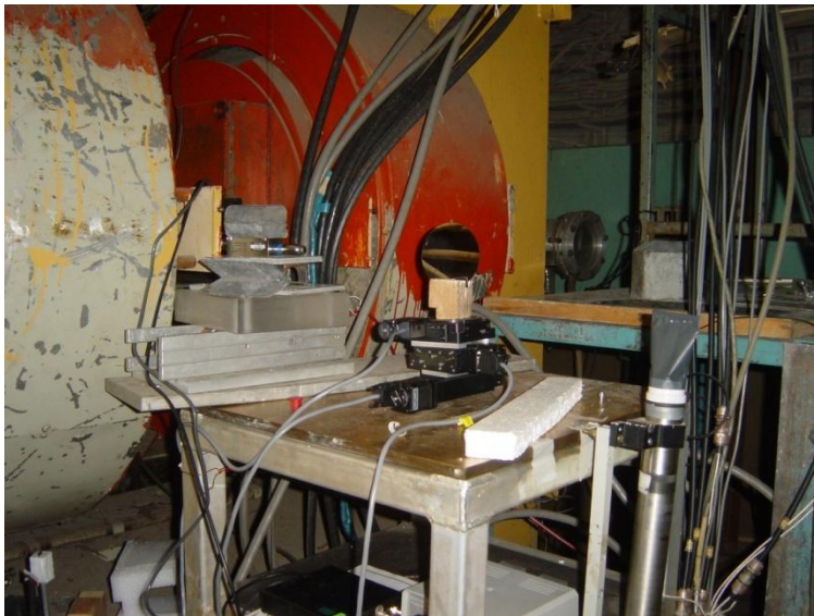
Fig. 5. The experimental setup for the PXR measurements
