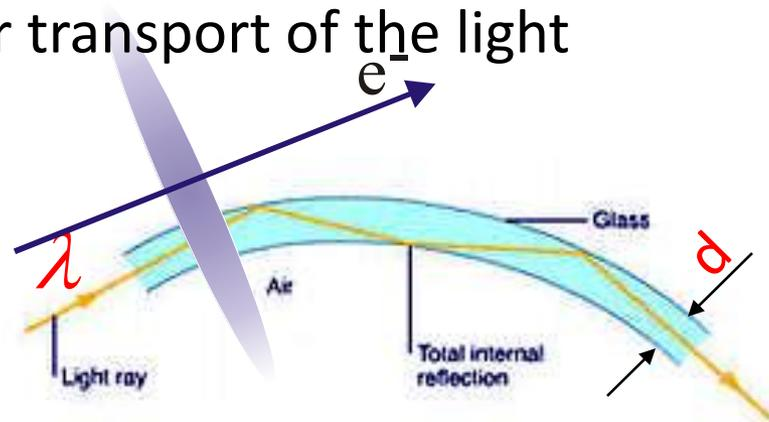
based on the full internal reflection in fiber.
