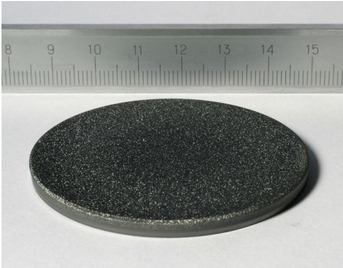
Photo diamond film grown on a silicon substrate with a diameter 57 mm.
