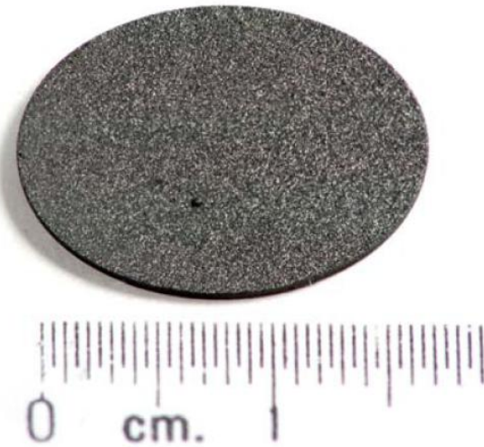
Photo of the target manufactured of the CVD-diamond without the silicon substrate with a diameter of 18 mm.
