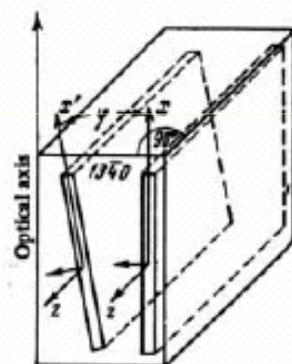
FIG. 4. Position of compared plates in the single-crystal quartz block.
