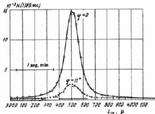
FIG. 5.  $K_{\alpha_1}$  Sn x-ray line obtained with a two-meter Cauchois spectrometer using compared plates of 1 mm thickness. Receiving slit  $\approx 250\mu$ ;  $N$  - number of  $\gamma$  quanta registered in 30 sec;  $l_{cr}$  - linear displacement of the end of the one-meter arm of the crystal drive. The vertical scale is doubled for the  $\varphi = 11^\circ$  line.
