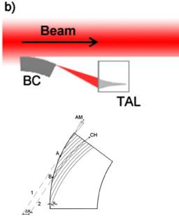
Using of bent crystal (BC) for beam collimation:
