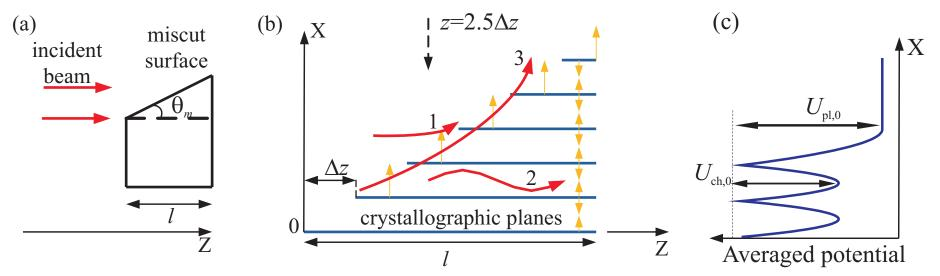
(a) Particles penetrates into the crystal through the lateral miscut surface;
