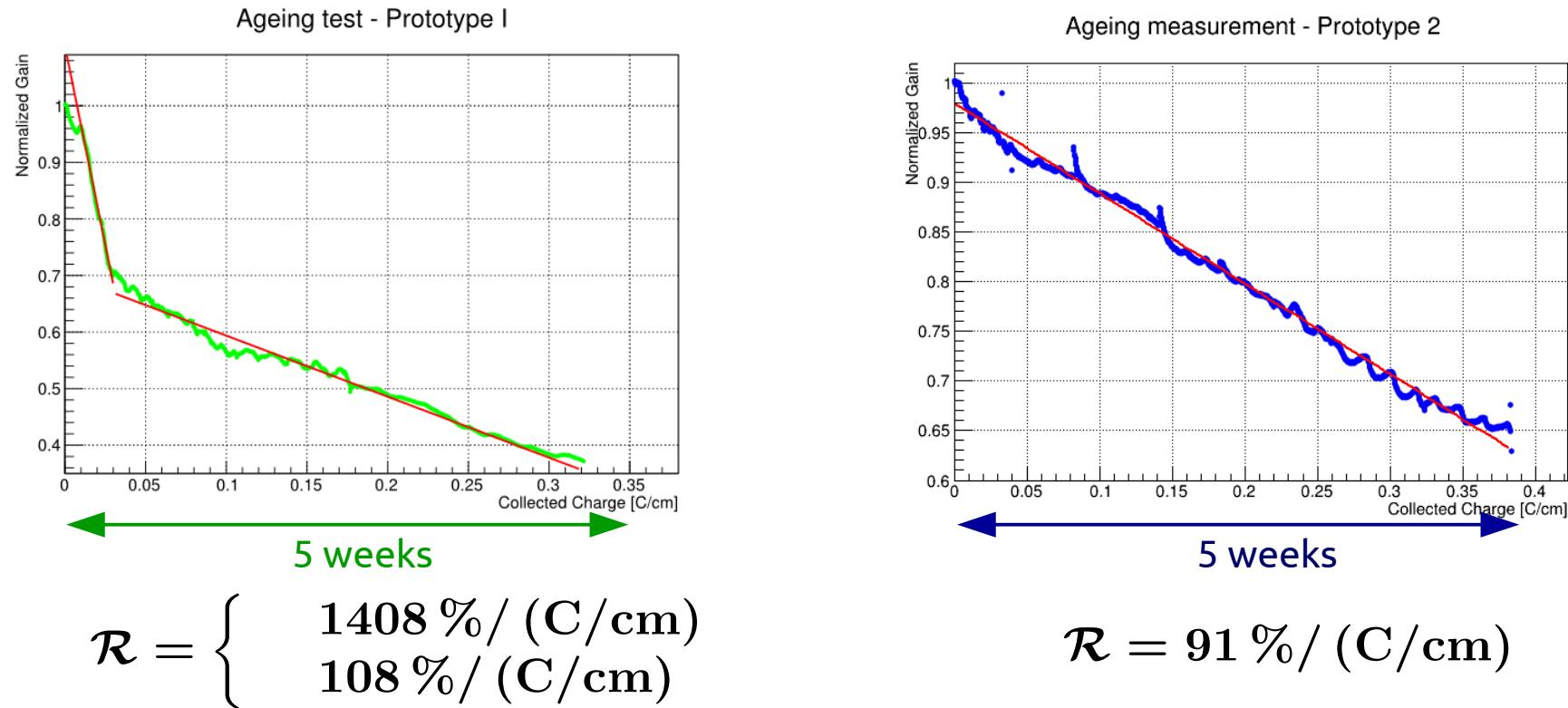
The measured ageing rates predict a **16% gain loss/year** in the hottest region of the chamber
