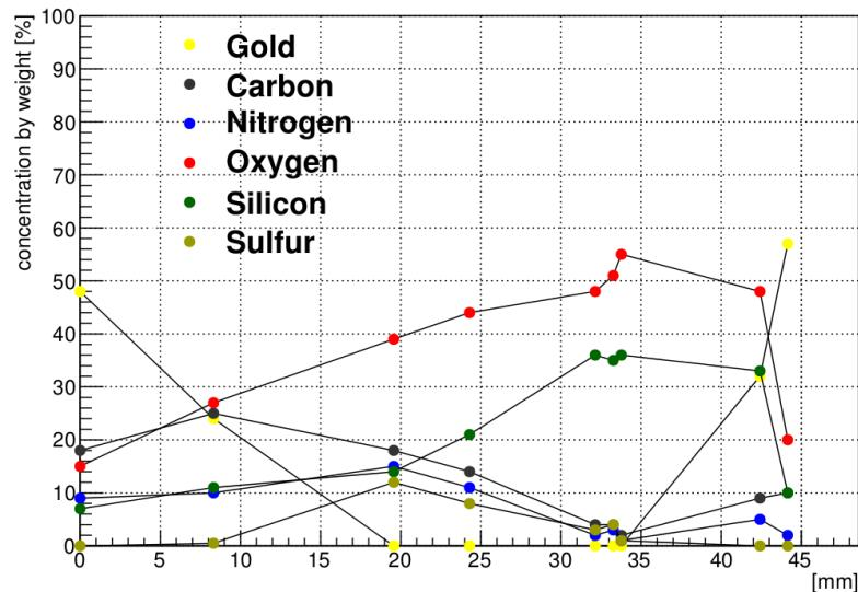
From EDX analysis a coated area with length  $\sim 3\text{ cm}$  is clearly visible.
