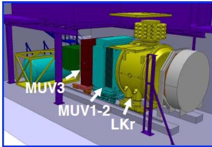
**MUV1-2: Fe/scintillator hadron calorimeter**
