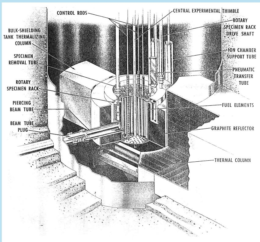
The core is placed at the bottom of the 6.25-m-high open tank with 2-m diameter.
