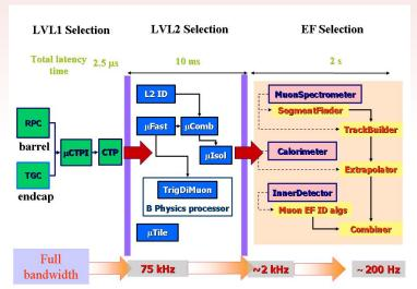
▶ Starting from next run L2 and EF will be merged in a High Level Trigger (HLT), combining various algorithms.
