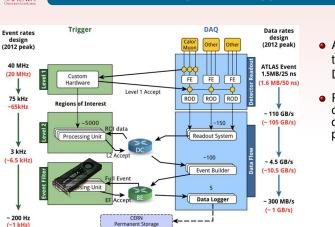
Atlas has implemented a three stage Trigger and DAQ system
