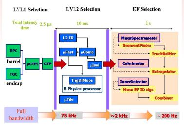
► Starting from next run L2 and EF will be merged in a High Level Trigger (HLT), combining various algorithms.
