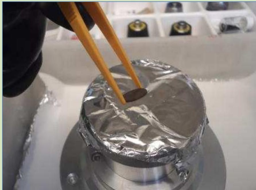
Starting point:  $\text{UO}_2$  of selected particle size ( $< 20 \mu\text{m}$ )
