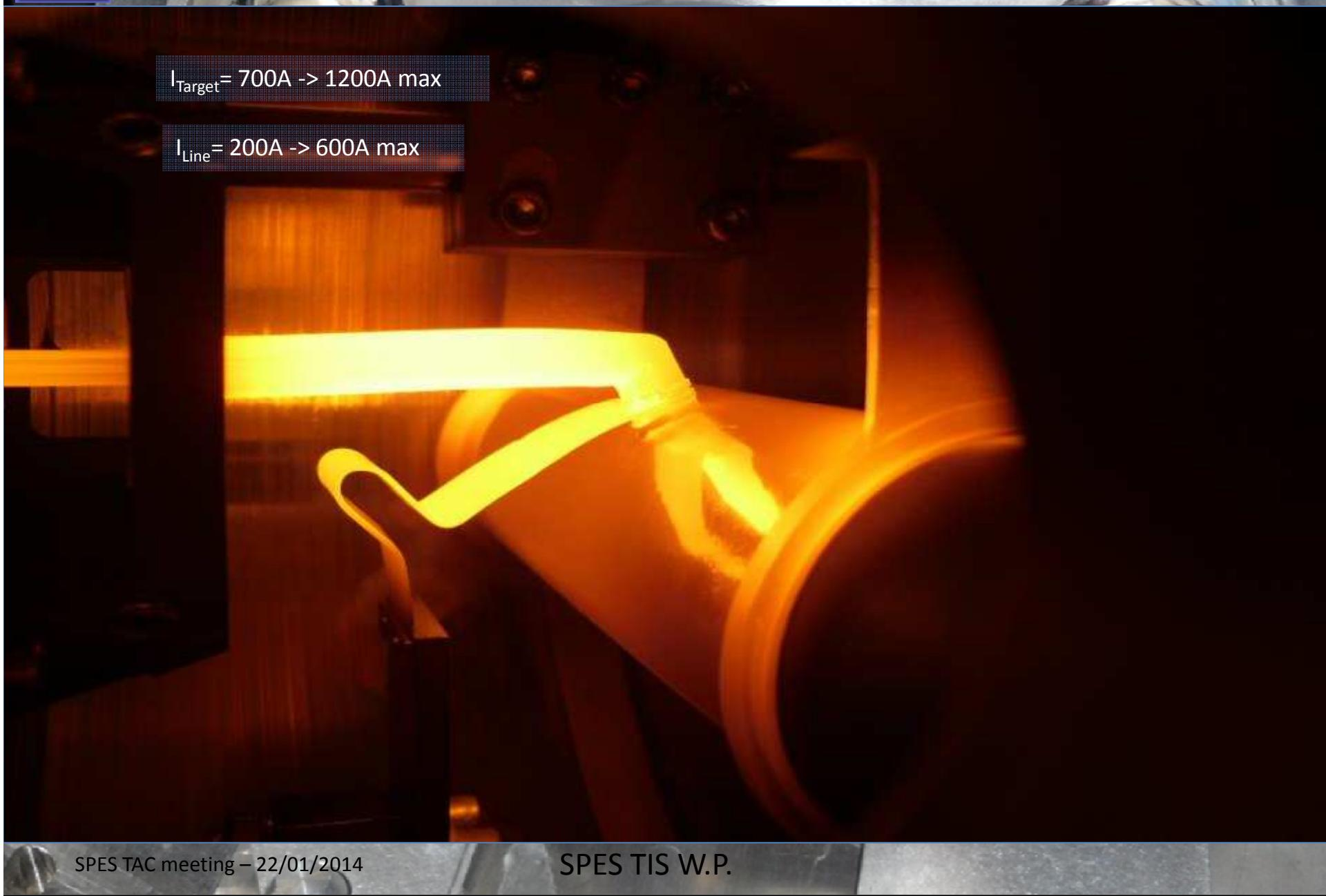
**high power testing ( $\approx 10$  kW) of the water-cooled target chamber**
