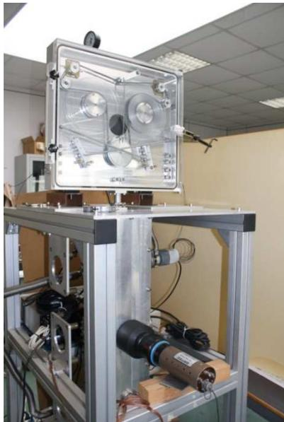
**Tape station system**: under development for SPES; moving tape system (1 cm wide mylar tape) and  $\gamma$ -ray counting chamber. Ge detectors, well shielded from potential background in the beam pipe, will be located at the counting chamber in a different position, a few cm far from the tape. The counting chamber will also accommodate plastic detectors for detecting positron decays.
