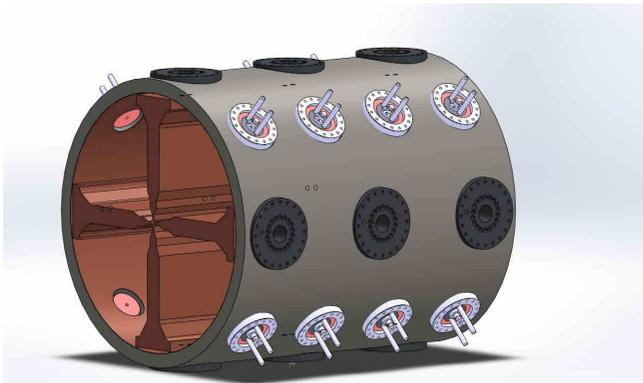
Mechanical layout of the RFQ tank module of about 1 meter.
