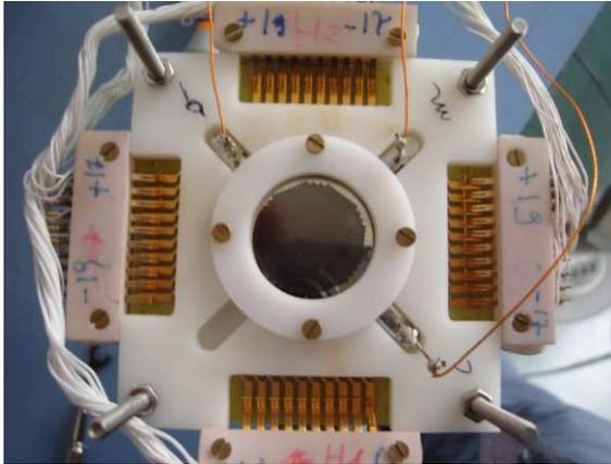
**Beam position and profile monitors**, based essentially on microchannel plates (MCP) as beam intensifiers. MCP is put directly on the beam line. Electrons produced on it and collected, after multiplication, on a position sensitive anode give the beam impact position. Measured 0.75 mm position resolution was measured for a 100 fA  $^{12}\text{C}$  beam. **FC, E,  $\phi$  detectors** are developed too.
