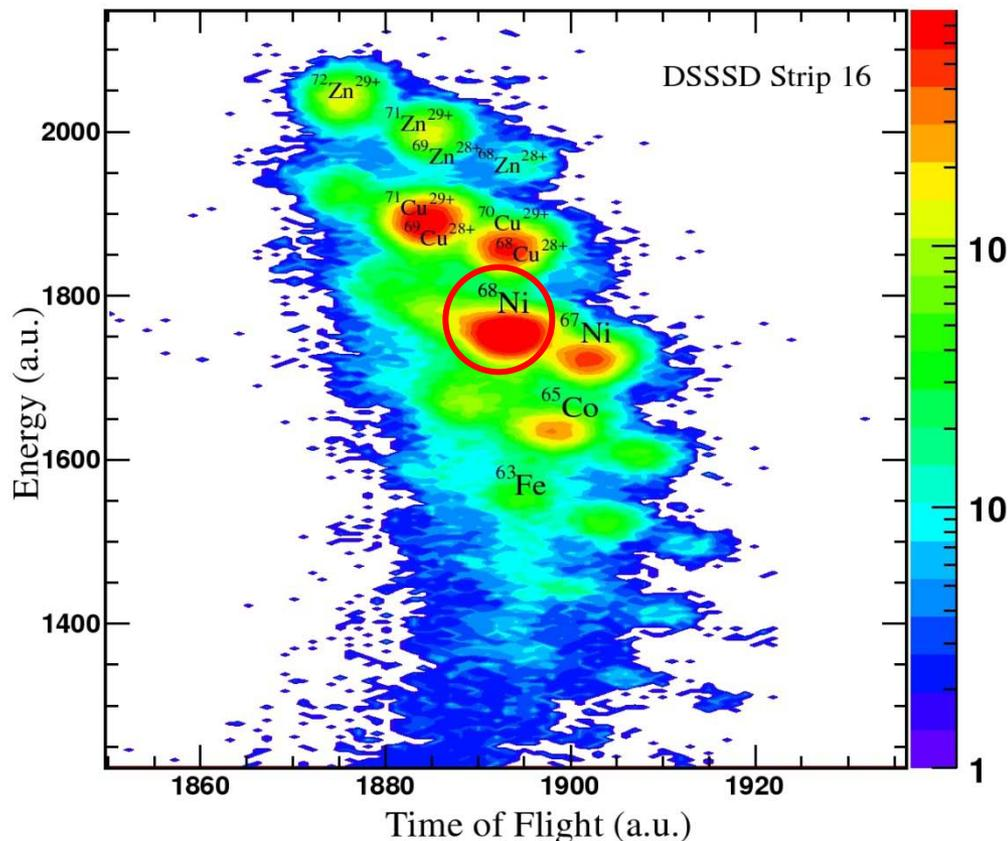
Production of a  $\approx 30$  A.MeV  $^{68}\text{Ni}$  beam at LNS (TimeScaleZn test)
