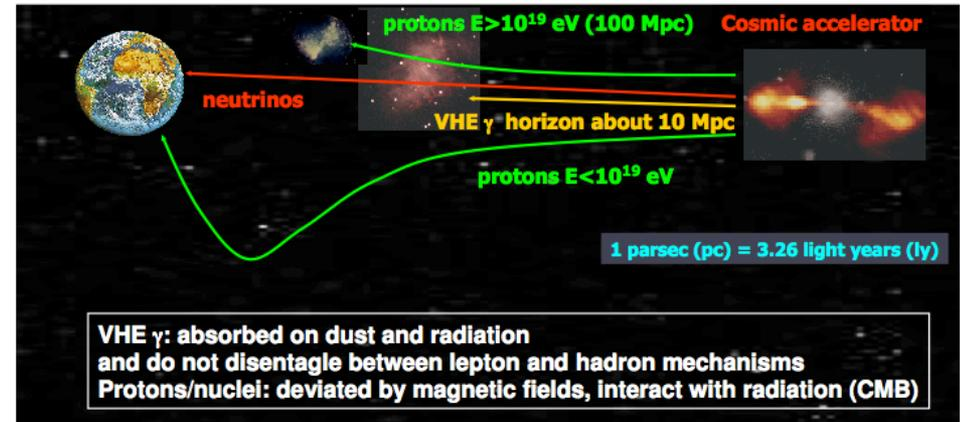
Neutrinos will provide unique pieces of information on the High Energy Universe. Detection possible by tracking the secondary muons in a km-cube size array of photosensors in deep sea waters
