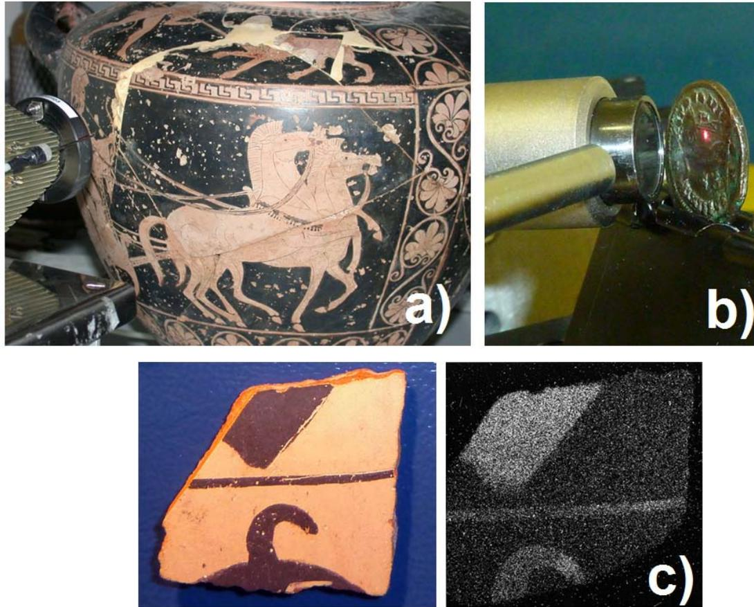
LANDIS collaboration: *innovative IBA (Ion Beam Analysis) and XRS (X-ray Spectrometry) non-destructive methods for in-situ applications in the Cultural Heritage field. The figure shows some complementary techniques – the PIXE-alfa, the LE-micro-XRF (low energy micro-XRF) and the X-ray imaging and space resolved spectroscopy – recently commissioned at the LANDIS laboratory for the analysis of surfaces in Arts and Archaeology.*
